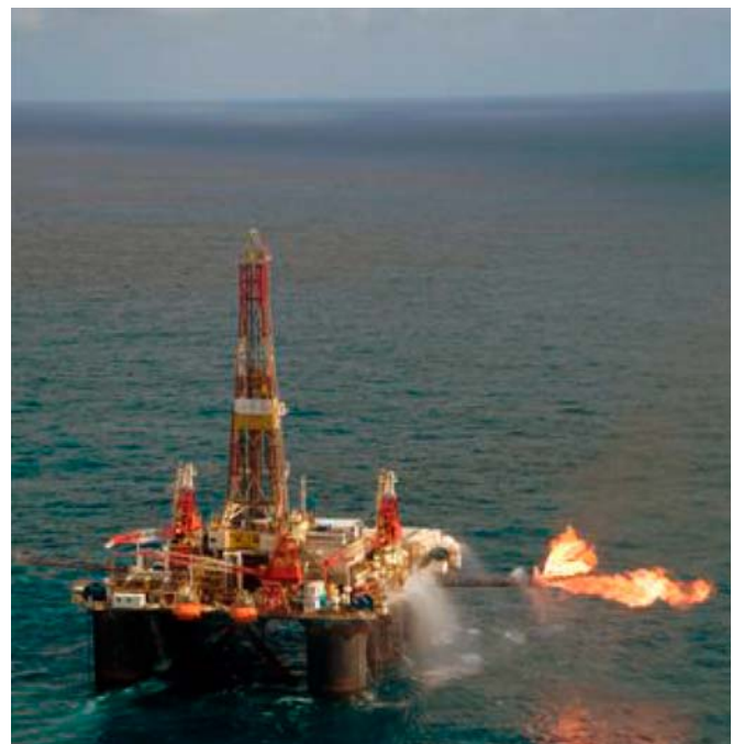
Kan Tan IV flow testing the Victory Discovery
